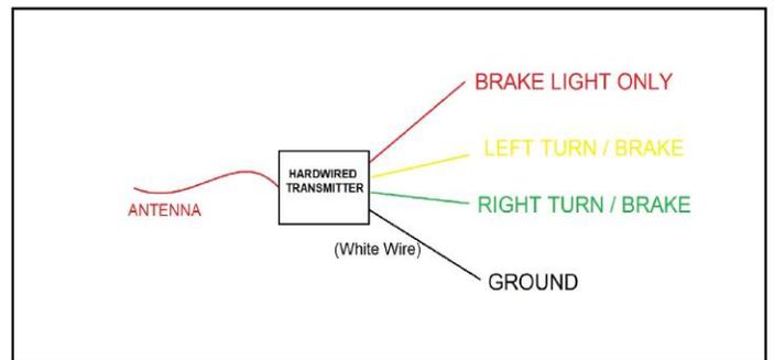
\*\* When testing for a ground circuit to connect the white wire on the transmitter we strongly recommend having all the lights turned on - This will prevent you from connecting to a floating ground (Which will cause crazy things to happen)
